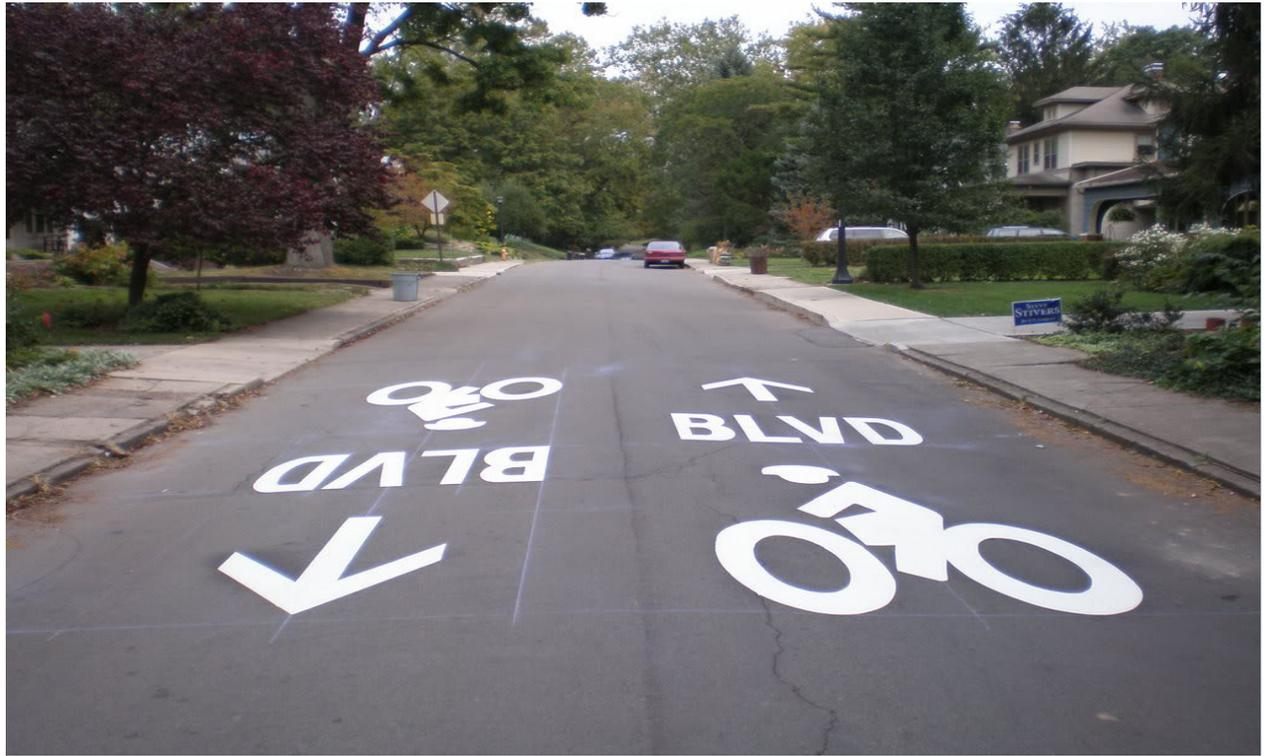
Use pavement markings along Bike Boulevards, spaced 250 feet apart. Photo credit: <http://www.columbusunderground.com/>
