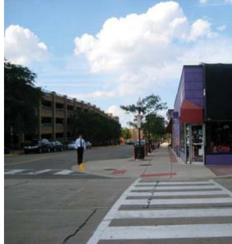
Example of a ladder-style crosswalk with bi-directional curb cuts and a curb extension.
